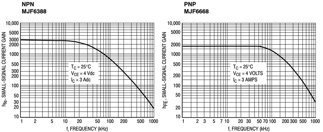
Figure 7. Typical Small-Signal Current Gain
