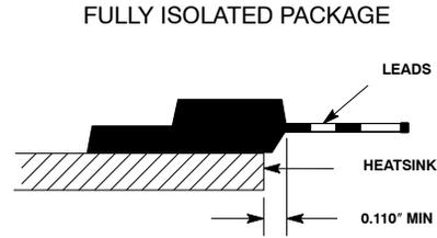
**Figure 14. Mounting Position**
