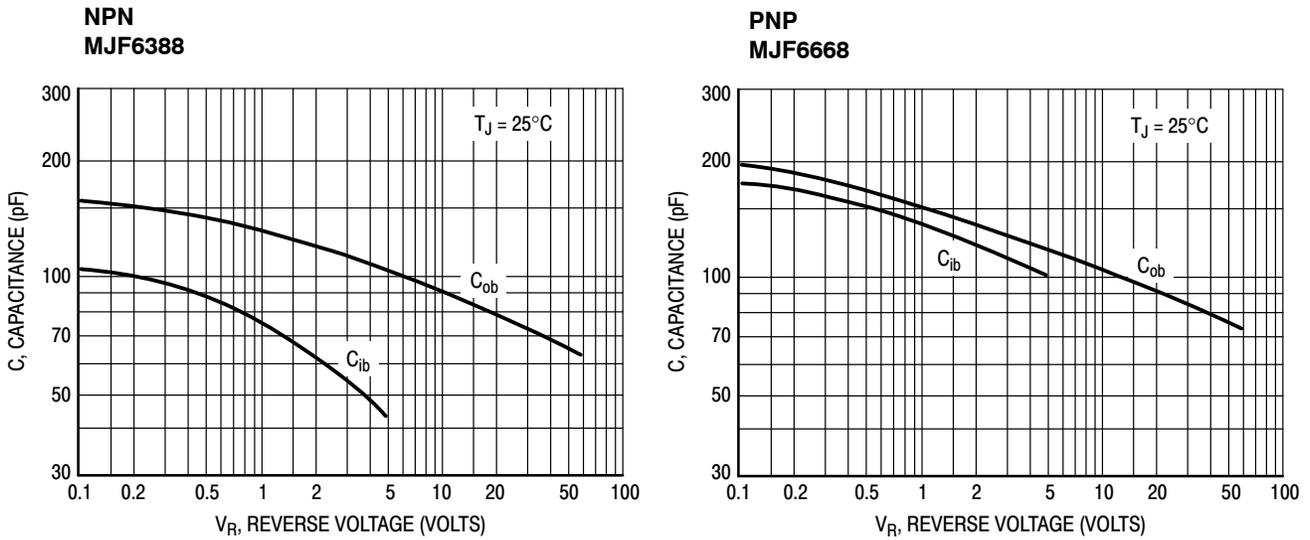
Figure 8. Typical Capacitance
