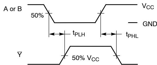
Figure 4. Switching Waveforms
