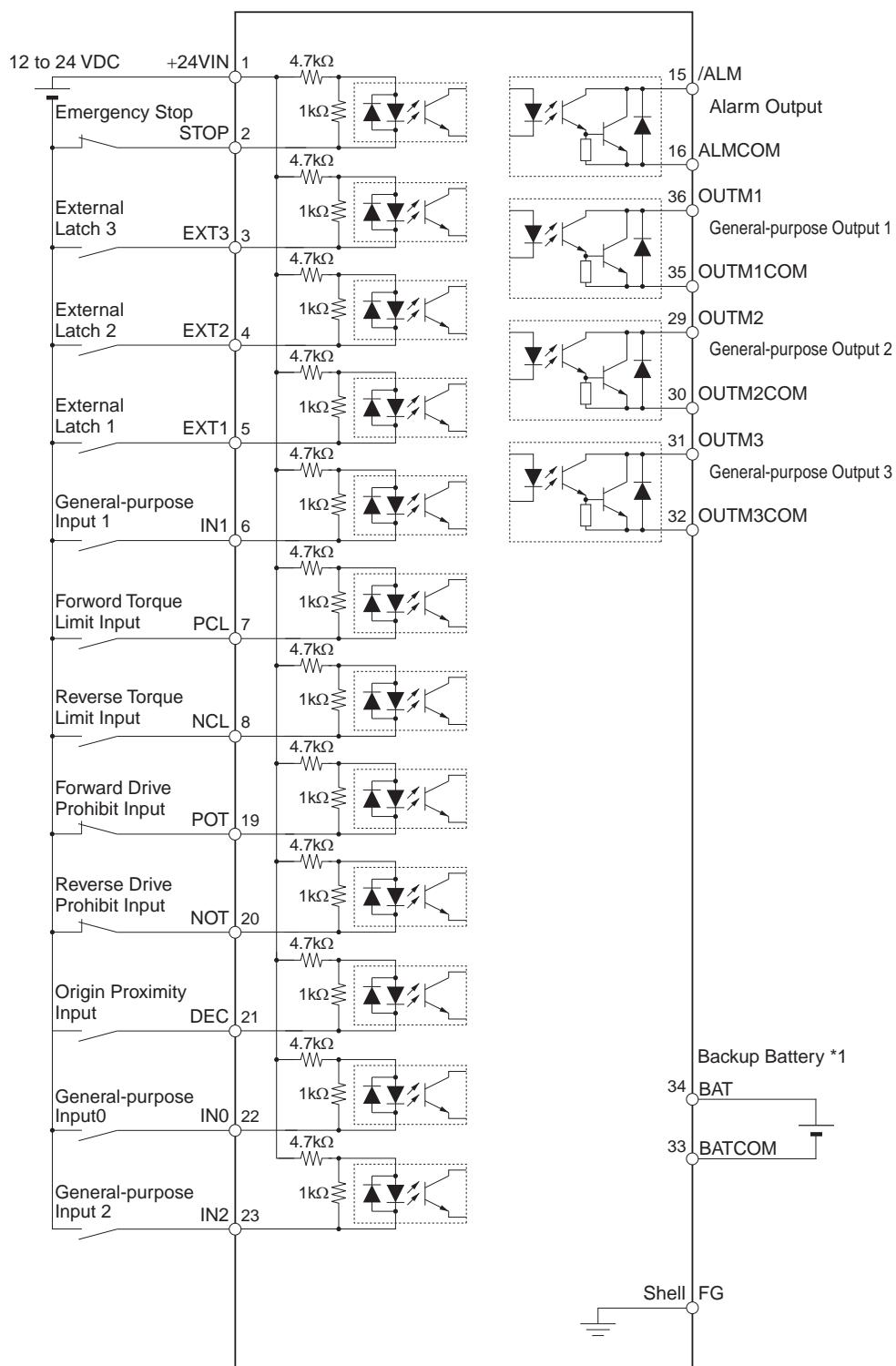
\*1. If a backup battery is connected, a cable with a battery is not required.
