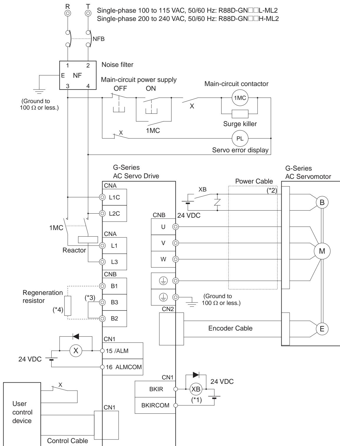
\*1. Recommended relay: MY Relay (24 V), by OMRON. For example, the MY2 Relay's rated inductive load is 2 A at 24 VDC and applicable to all G-Series Servomotors with brakes.
