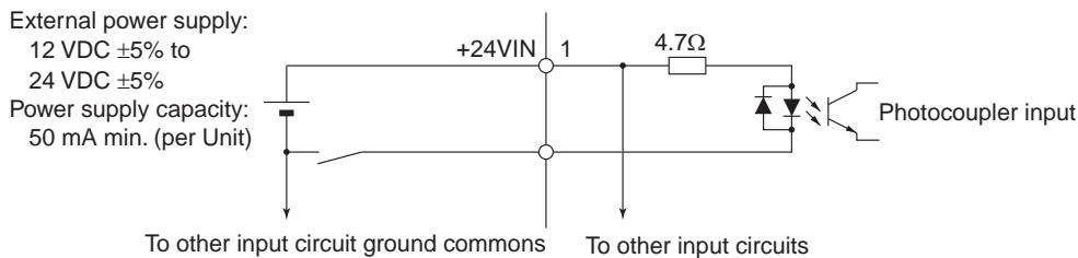
Signal Levels    ON level: 10 V min.
