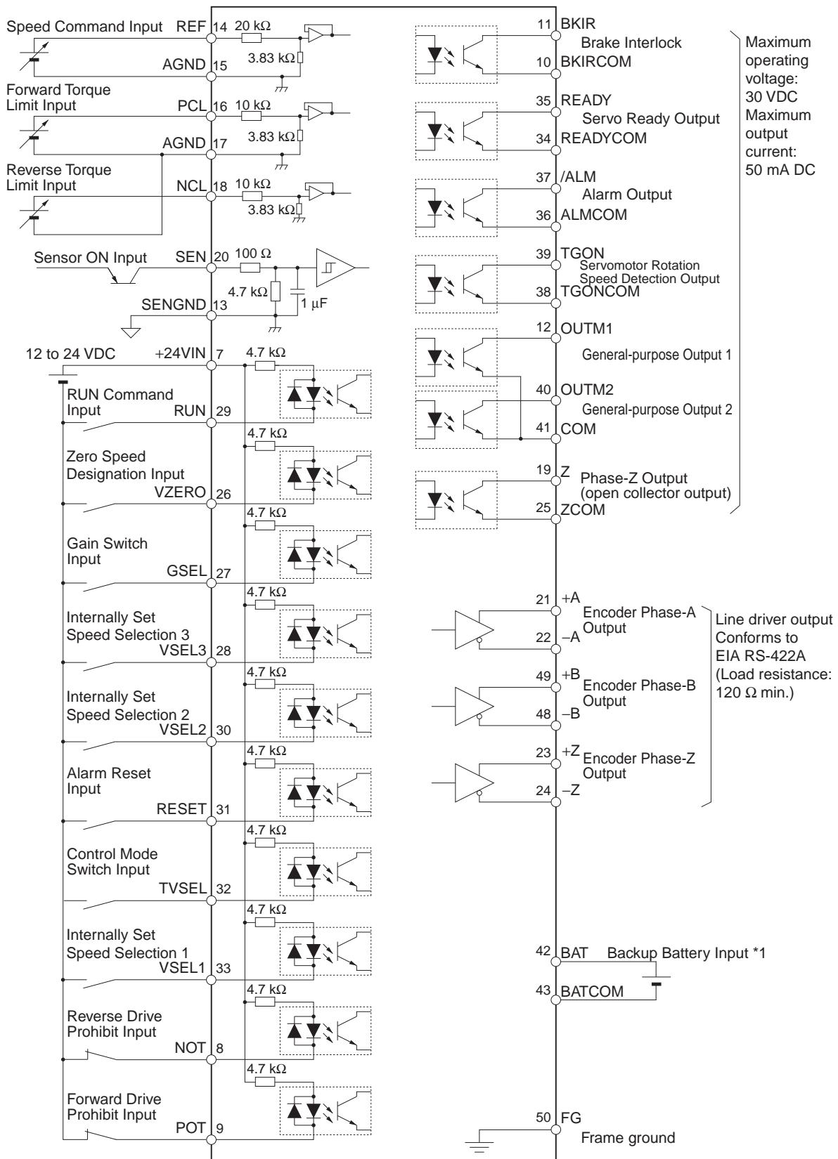
\*1. If a backup battery is connected, a cable with a battery is not required.
