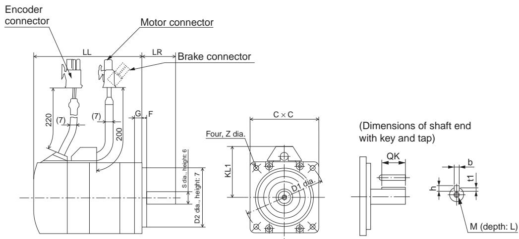
**2,000-r/min Cylindrical Servomotors**
