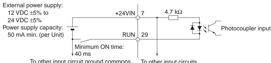
Signal Levels    ON level: 10 V min.
