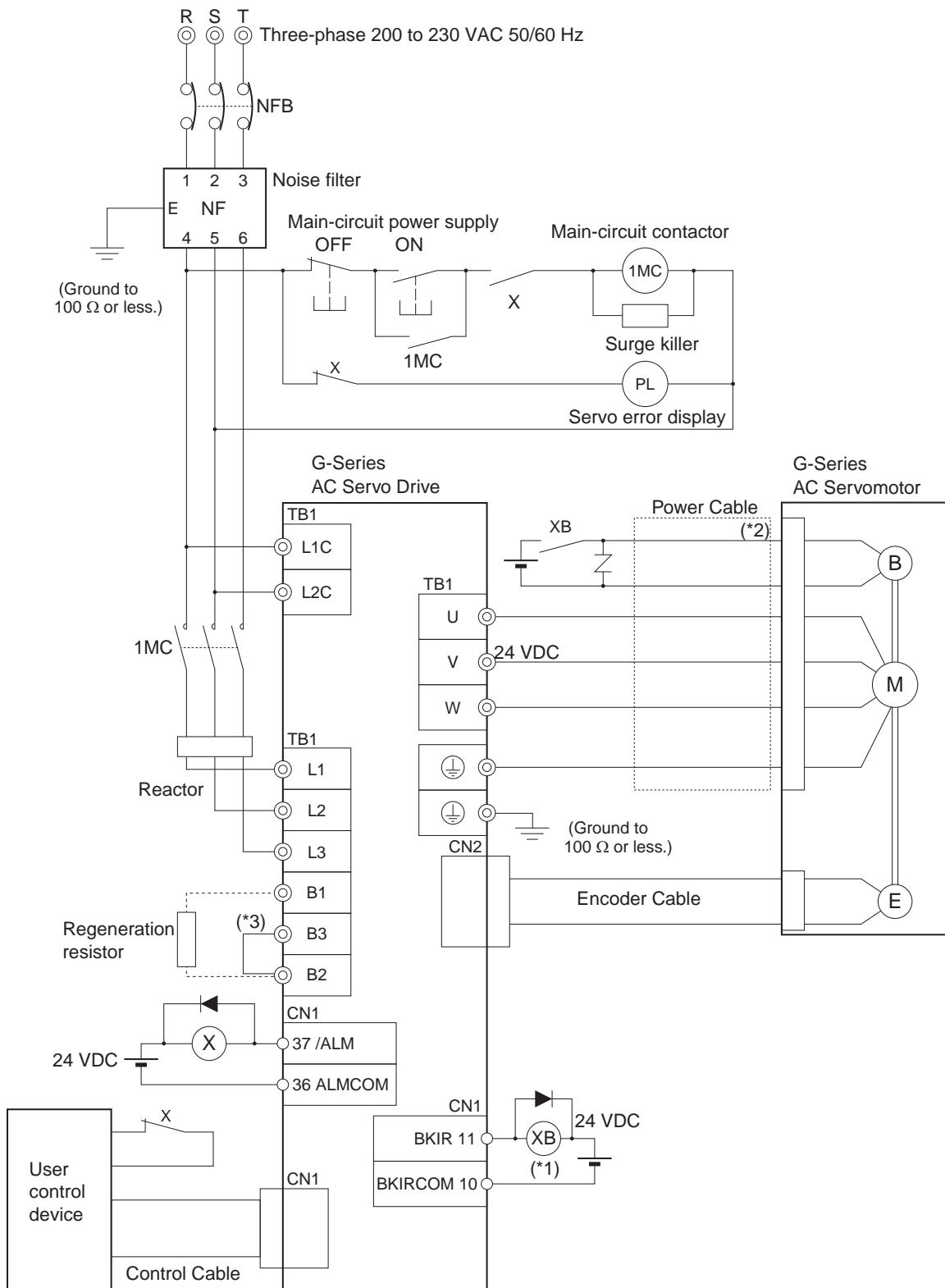
\*1. Recommended relay: MY Relay (24 V), by OMRON. For example, the MY2 Relay's rated inductive load is 2 A at 24 VDC and applicable to all G-Series Servomotors with brakes.
