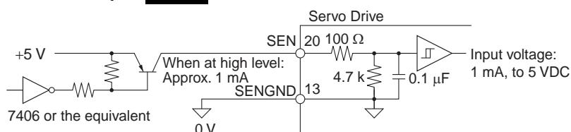
Signal Levels    High level: 4 V min.
