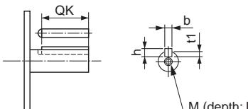
**Note:** The standard models have a straight shaft. A model with a key and tap is indicated by adding "S2" to the end of the model number.
