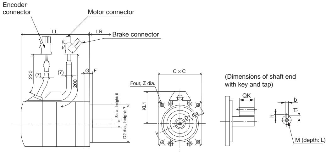
**2,000-r/min Cylindrical Servomotors**
