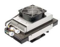
The AA Outdoor Cooler Series is an air-to-air thermoelectric assembly (TEA) that uses impingement flow to transfer heat. It offers dependable, compact performance by cooling objects via convection. Heat is absorbed and dissipated thru high density heat exchangers equipped with air ducted shrouds and brand name fans. The heat pumping action occurs from custom designed thermoelectric modules that achieve a high coefficient of performance (COP) to minimize power consumption.
