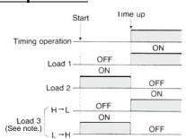
Note: Output transistor ON: Low (0 V) Output transistor OFF: High (12 V)
