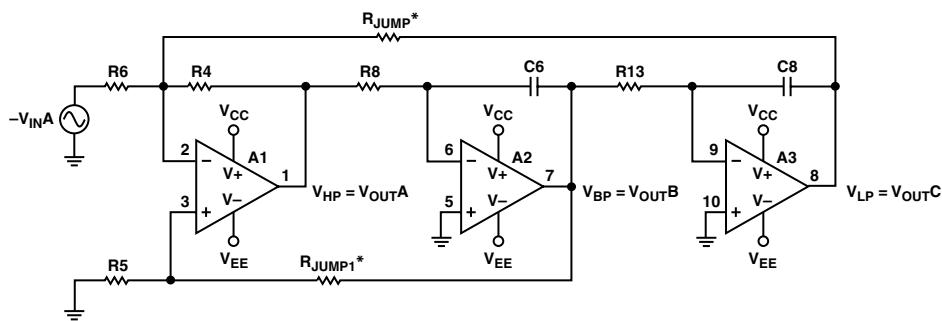
\* $R_{JUMP}$  AND  $R_{JUMP1}$  IS AN EXTERNAL COMPONENT, NOT PROVIDED ON THE APPLICATION BOARD.
