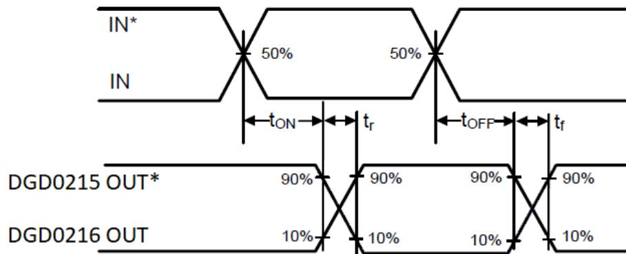
**Figure 1.** Switching Time Waveform Definitions
