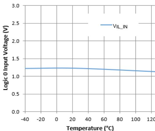
Figure 19. Logic 0 Input Voltage vs. Temperature
