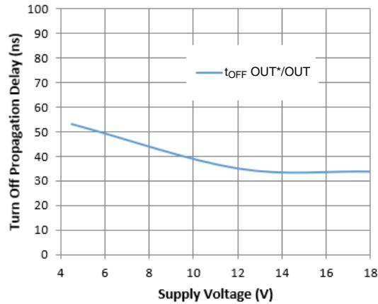
**Figure 4.** Turn-off Propagation Delay vs. Supply Voltage
