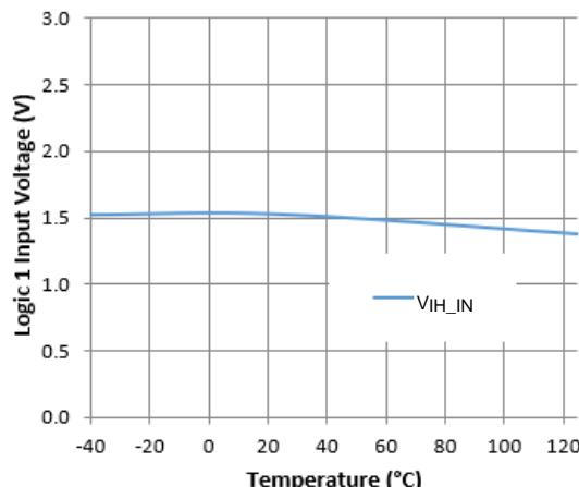
Figure 17. Logic 1 Input Voltage vs. Temperature
