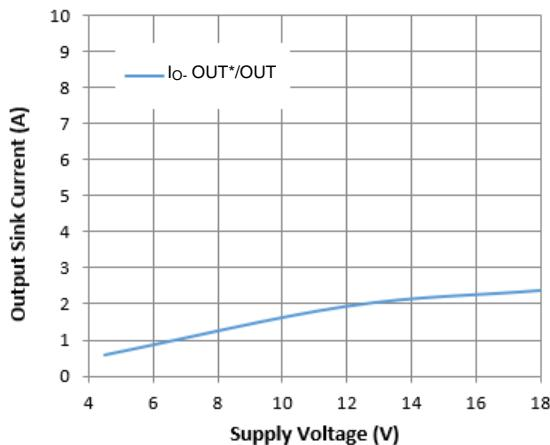
Figure 14. Output Sink Current vs. Supply Voltage
