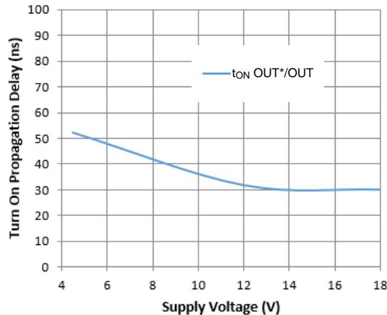
**Figure 2.** Turn-on Propagation Delay vs. Supply Voltage
