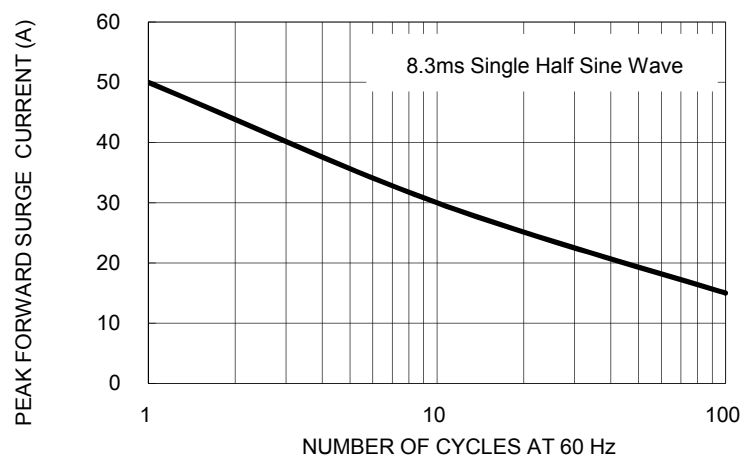
FIG. 3 MAXIMUM NON-REPETITIVE FORWARD SURGE CURRENT
