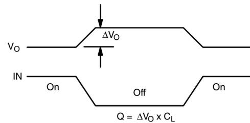
Figure 4. Charge Injection
