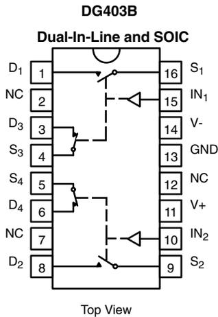
Four SPST Switches in Two Pairs per Package
