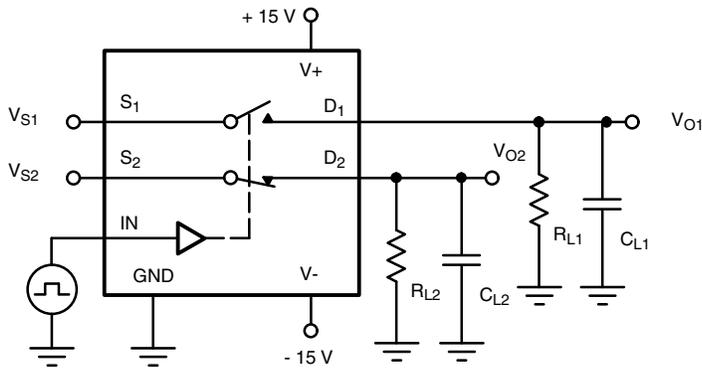
$C_L$  (includes fixture and stray capacitance)
