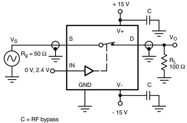
Figure 6. Insertion Loss
