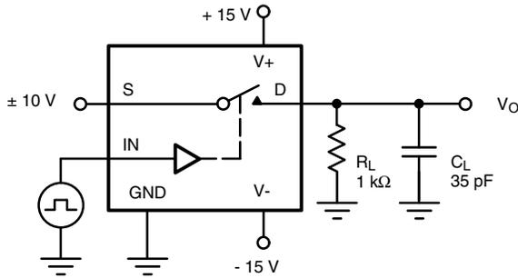
$C_L$  (includes fixture and stray capacitance)
