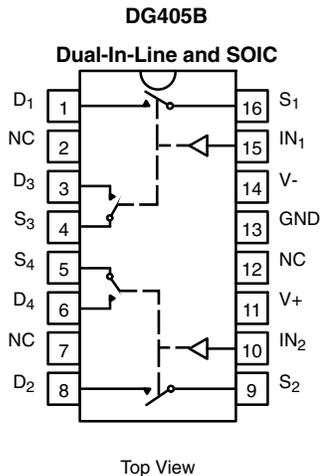
Four SPST Switches in Two Pairs per Package
