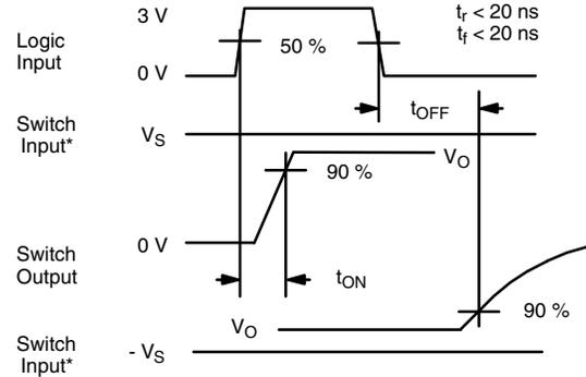
\*  $V_S = 10\text{ V}$  for  $t_{ON}$ ,  $V_S = -10\text{ V}$  for  $t_{OFF}$
