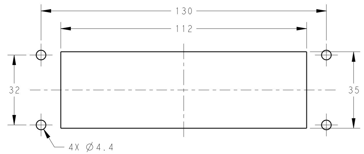
T1425240000-000 H24B-AG-BO-EMC H24B EMC HOUSING, BULKHEAD MOUNTED, 4 EAR, NO LOCKING
