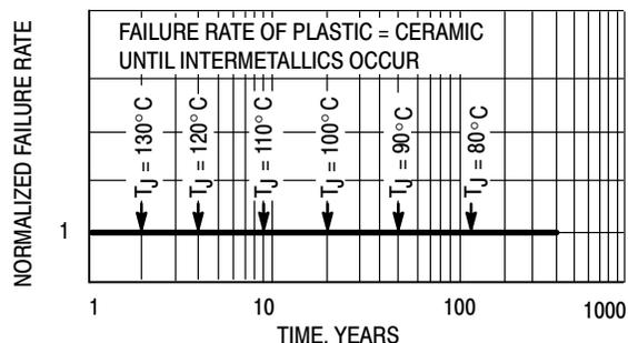
Figure 3. Failure Rate vs. Time Junction Temperature
