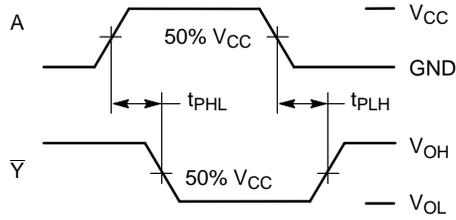
**Figure 4. Switching Waveforms**
