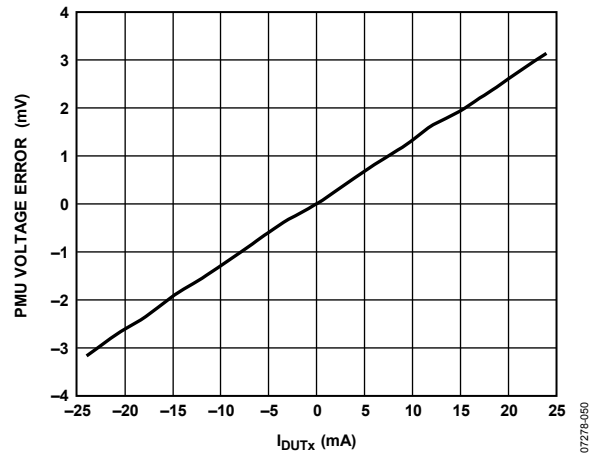
Figure 56. PMU Force Voltage Range A Output Voltage Error at 6.0 V vs. Output Current
