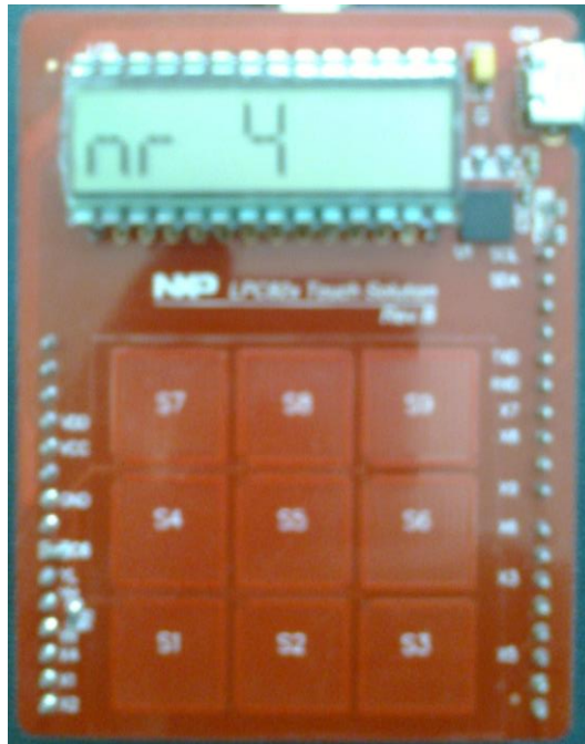
Fig 6. Gesture recognition by LPC824 target
