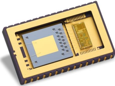
Figure 32 : Inner view of the package, showing the MEMS and IC
