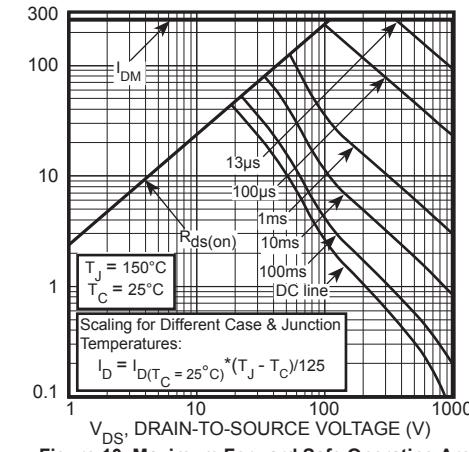
Figure 10, Maximum Forward Safe Operating Area
