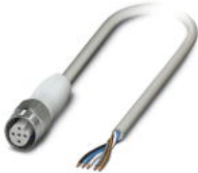
Sensor/Actuator cable, 5-position, PP-EPDM halogen-free, Gray RAL 7035, Free cable end, on Socket straight M12, A-coded, Cable length: 3 m, Hygienic design, With high-grade steel knurl
