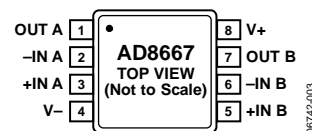
Figure 3. 8-Lead MSOP (RM-8), 8-Lead SOIC (R-8)
