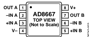
Figure 3. 8-Lead MSOP (RM-8), 8-Lead SOIC (R-8)
