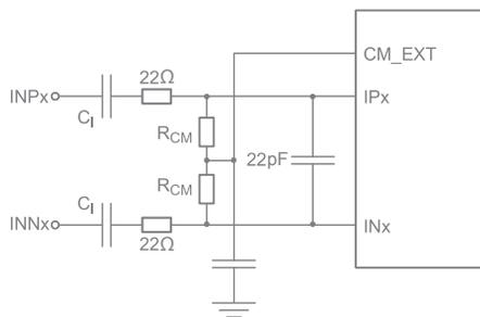
Figure 5. AC-Coupled Input
