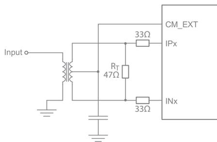
Figure 4. Transformer-Coupled Input
