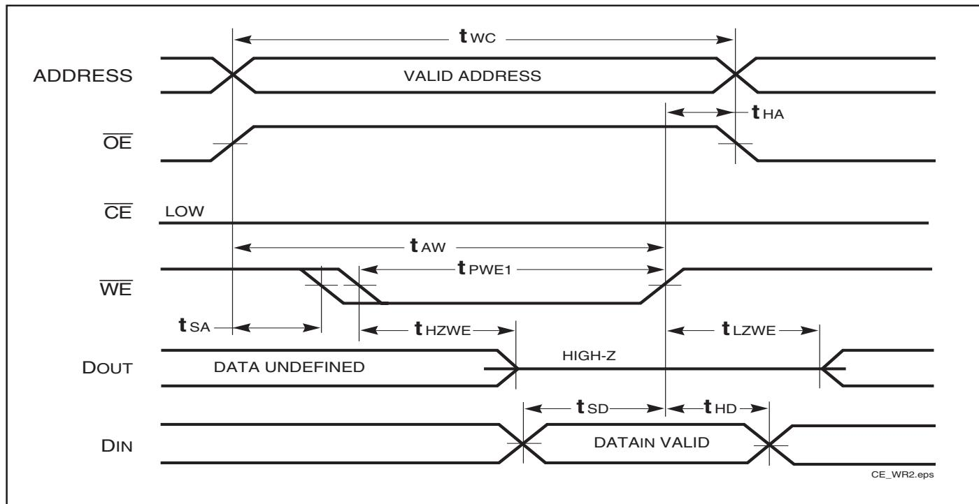
WRITE CYCLE NO. 3 ( $\overline{OE}$  is LOW During Write Cycle) <sup>(1)</sup>
