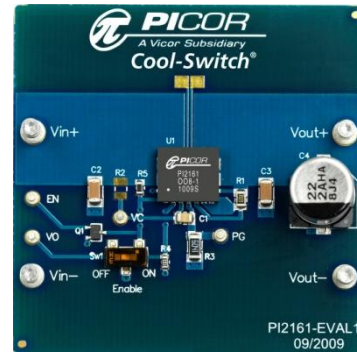
Figure 1: PI2161-EVAL1 Evaluation Board (1.8" x 1.8")
