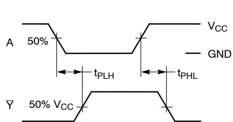
Figure 3. Switching Waveforms
