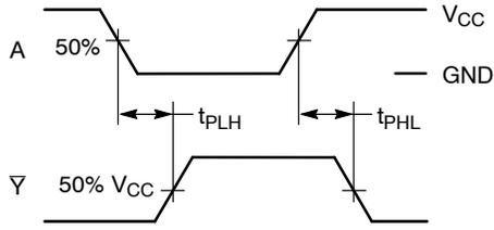
Figure 3. Switching Waveforms
