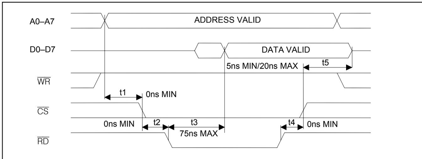
**Figure 26-5. Intel Bus Write Timing (PBTS = 0)**
