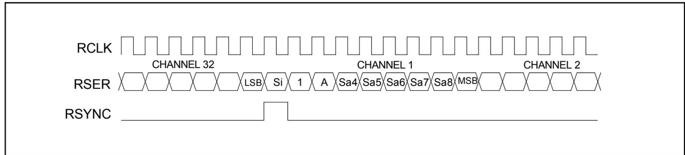
**Figure 24-3. Receive Boundary Timing (With Elastic Store Enabled)**
