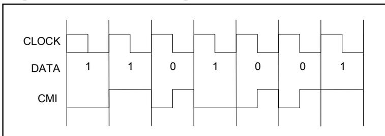
Transmit and receive CMI is enabled through OUTAC.7. When this register bit is set, the TTIP pin outputs CMI-coded data at normal TTL-type levels. This signal can be used to directly drive an optical interface. When CMI is enabled, the user can also use HDB3 coding.
