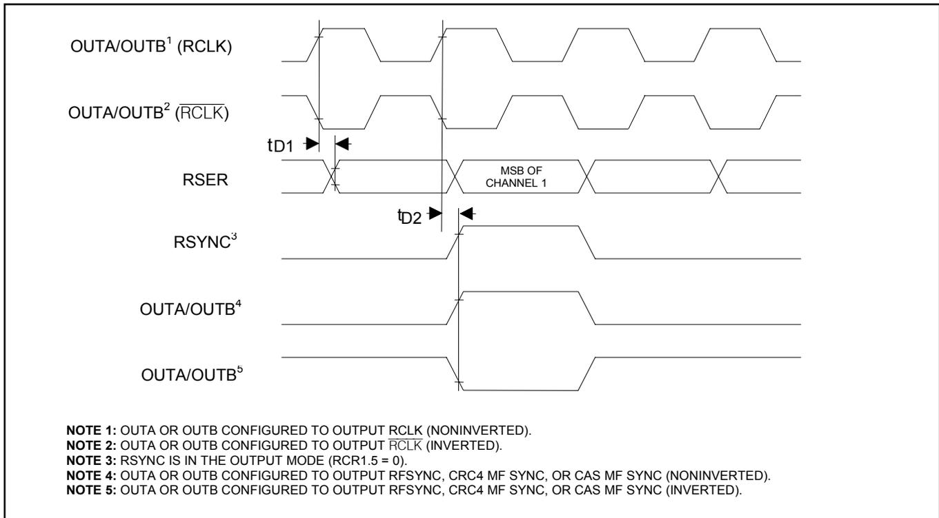
**Figure 26-10. Receive AC Timing (Receive Elastic Store Enabled)**
