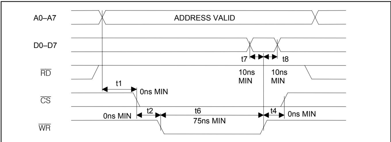
**Figure 26-6. Motorola Bus Read Timing (PBTS = 1)**
