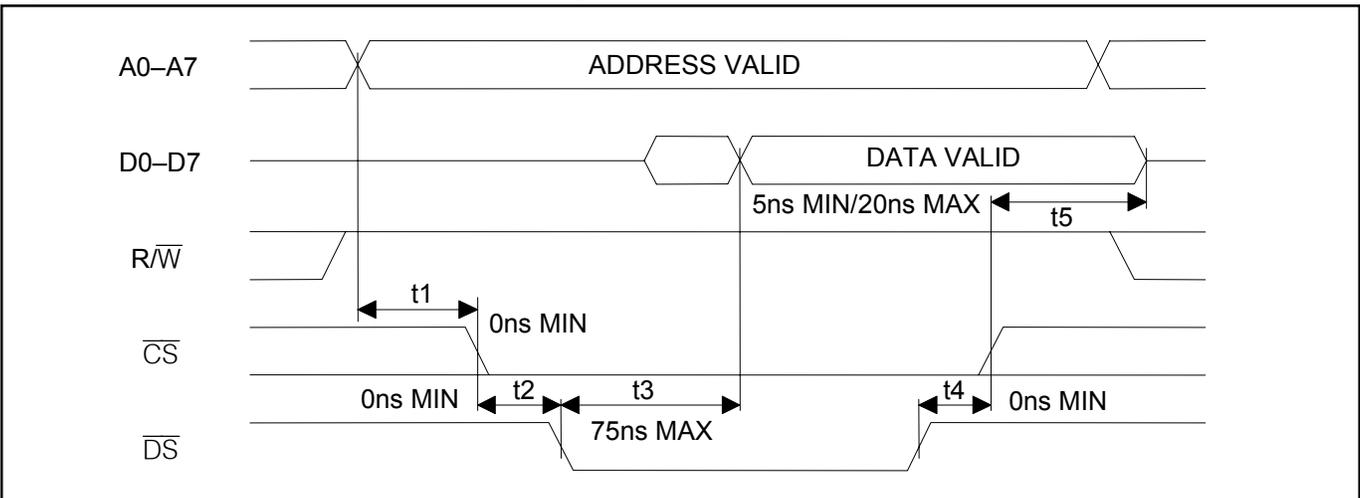
**Figure 26-7. Motorola Bus Write Timing (PBTS = 1)**
