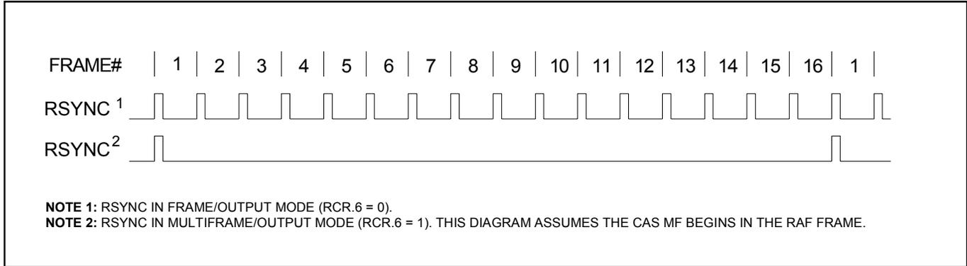
**Figure 24-2. Receive Boundary Timing (With Elastic Store Disabled)**
