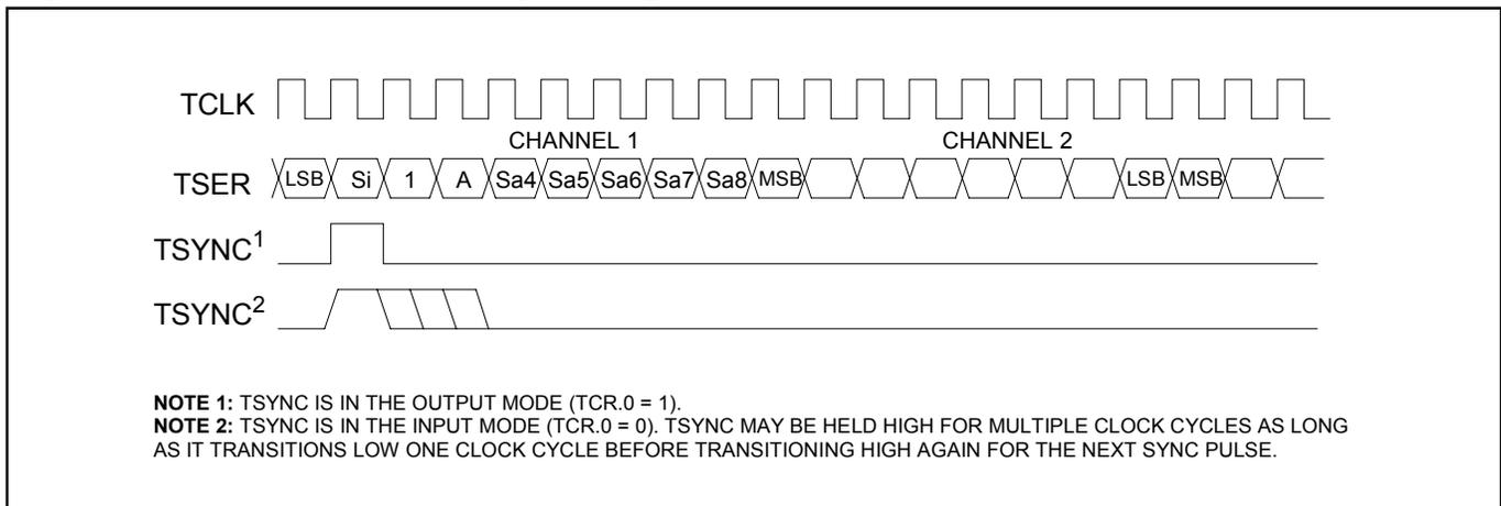
Figure 24-7. Transmit Interleave Bus Operation
