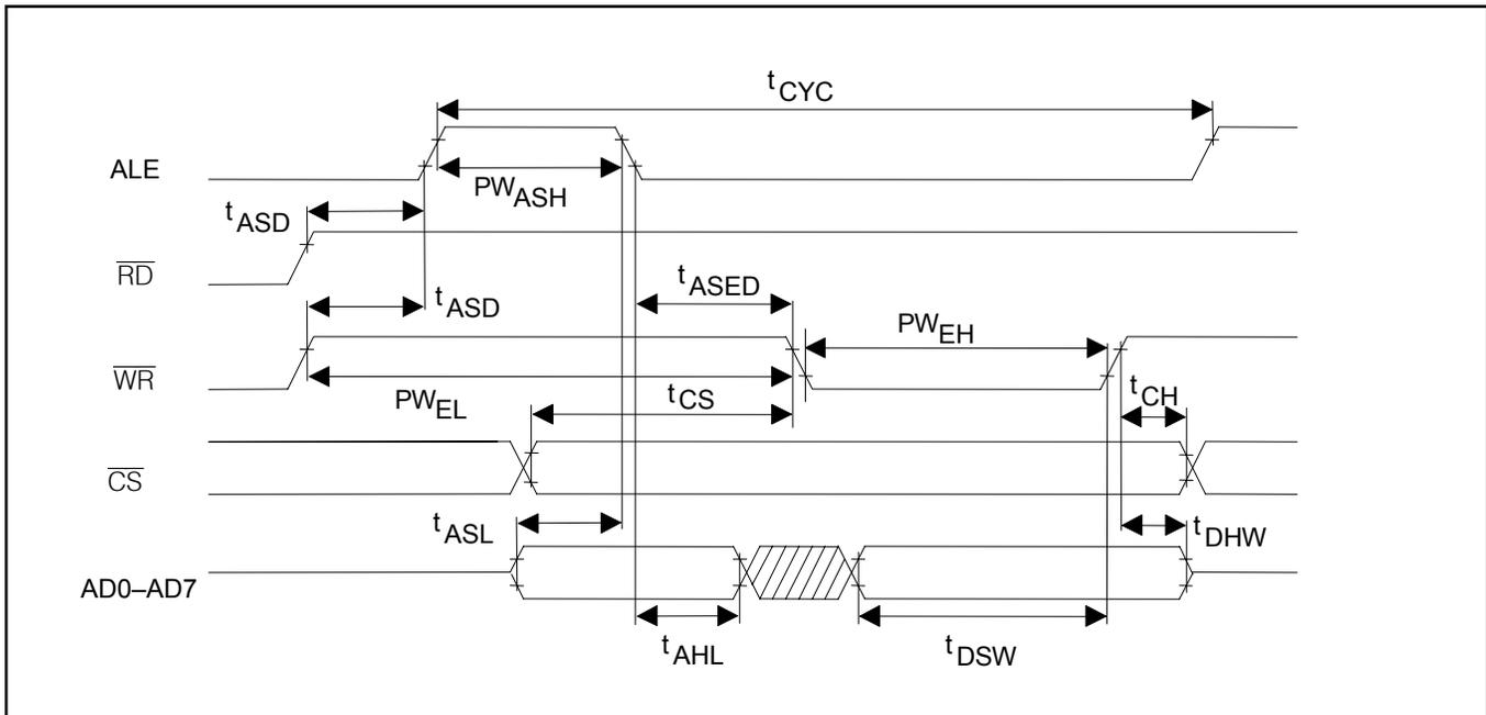
Figure 26-3. Motorola Bus AC Timing (PBTS = 1)
