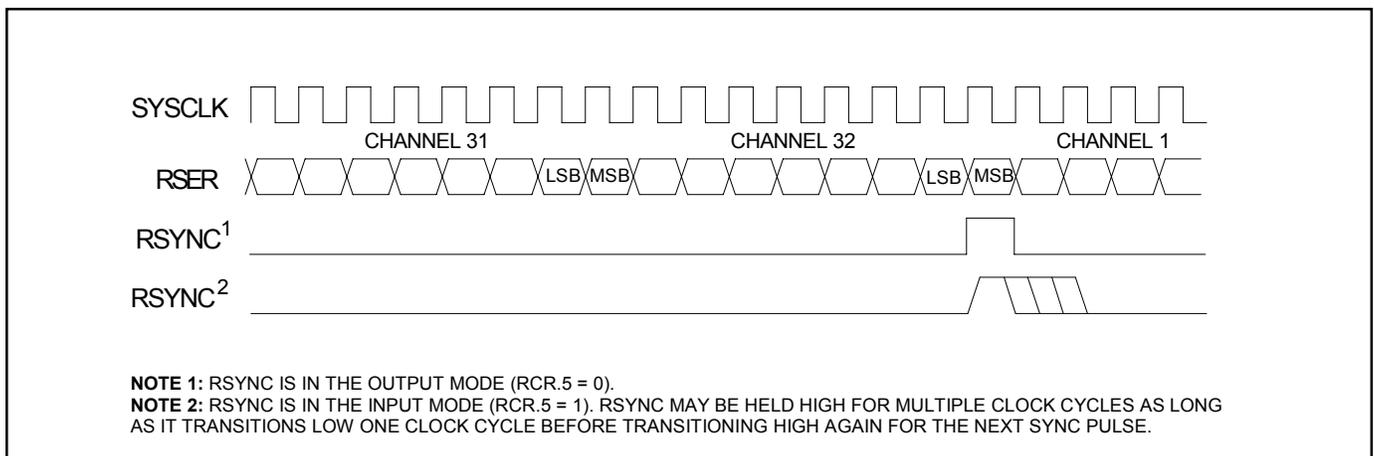
**Figure 24-4. Receive Interleave Bus Operation**
