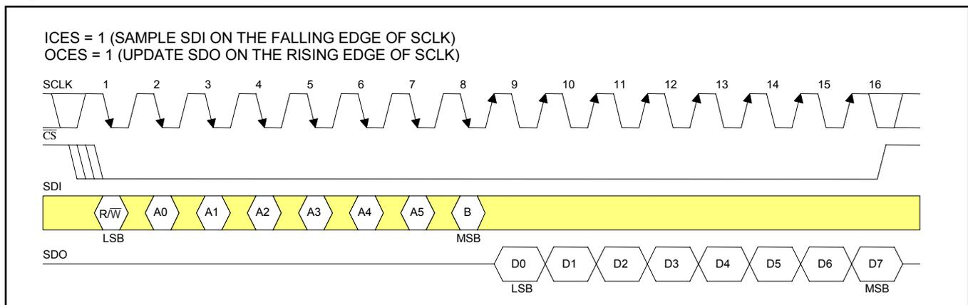
**Figure 6-2. Serial Port Operation Mode 2**
