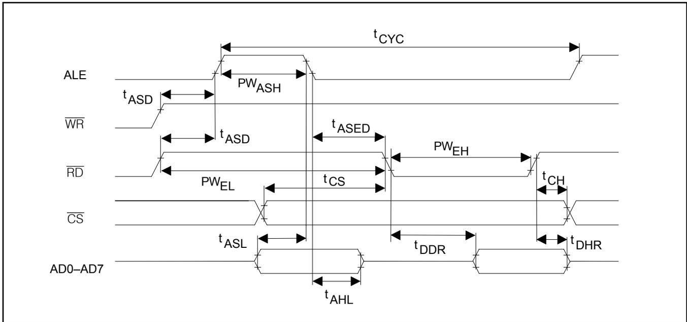
Figure 26-2. Intel Bus Write Timing (PBTS = 0)
