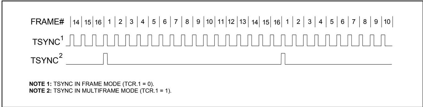
**Figure 24-6. Transmit Boundary Timing**
