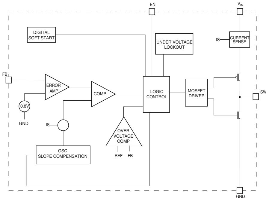
**Figure 4. Block Diagram**
