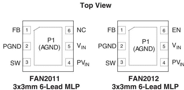
**Figure 2. Pin Assignment**
