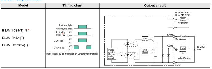
Note: Connect terminal 1 to any polarity and terminal 2 to the power supply because there is no polarity on the Emitter side.
