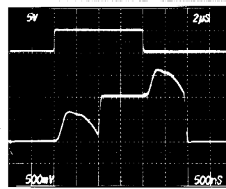
MUX-08 SMALL-SIGNAL SWITCHING WITH 2μs SAMPLE TIME
