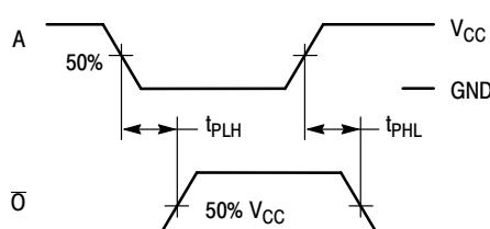
**Figure 3. Switching Waveforms**
