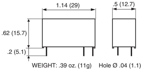
Figure 1 — TS relays; dimensions in inches (mm)
