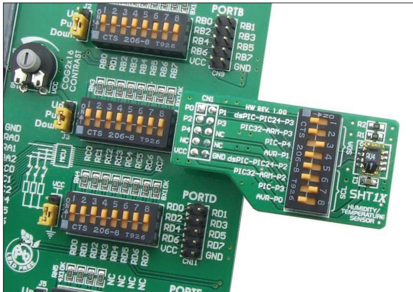
Figure 4: Additional board connected to a development system
