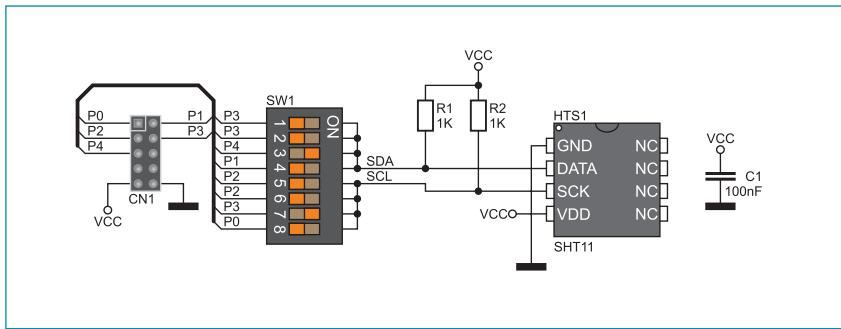
Figure 2: SHT1X additional board connection schematic
