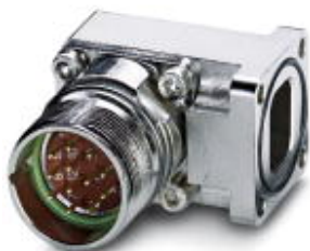
Device connector, front mounting, angled fixed, Screw locking, M23, number of positions: 17, type of contact: Pin, Crimp connection, Axial O-ring, 4x Ø 3.2, shielded: yes, flange dimensions: 26 mm x 26 mm
