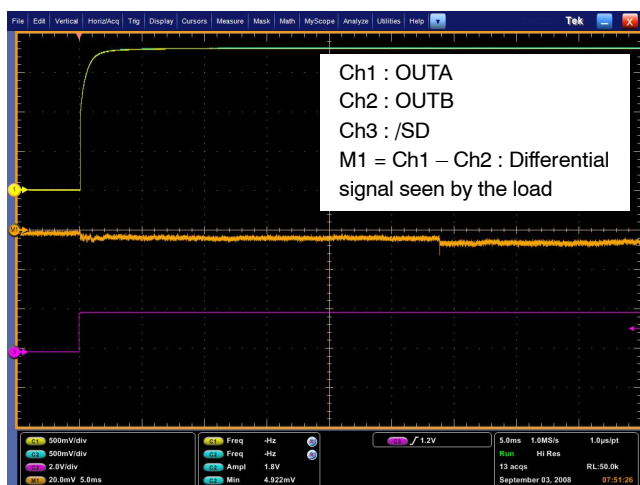
Figure 29. Zero pop noise turn on sequence with differential input to ground ( C_i = 100 \text{ nF} , R_i = 24 \text{ k}\Omega , R_f = 24 \text{ k}\Omega , C_{byp} = 1 \text{ }\mu\text{F} , R_l = 8 \text{ }\Omega , T_{on} = \text{GND} )
