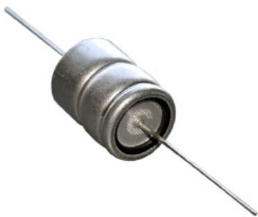
Type AXLH capacitors are a new generation of high performance aluminum electrolytic capacitors rated up to 2000 hours at 150 °C. They are designed for applications that place high demands on a capacitor. The capacitor's outstanding features include low ESR, low leakage current, a long shelf life and a high ripple current capability.
