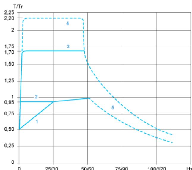
1 : Self-cooled motor: continuous useful torque
