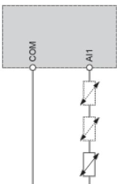
It is possible to connect either 1 or 3 sensors on terminals AI1.
