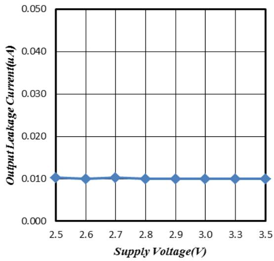
**Figure 7. Output Leakage Current vs. Supply Voltage**
