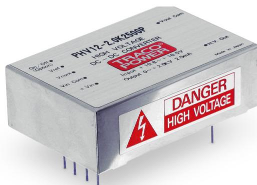
The PHV series are regulated miniature high voltage power modules using SMD and hybrid technology. They are designed for PCB mounting. The use of high stability components guarantees a minimal temperature drift and a very stable output voltage. Typical applications for these HV power supplies are photomultiplier tubes, gas chromatography, analytical instruments and wherever where small size and high output voltage stability is requested.
