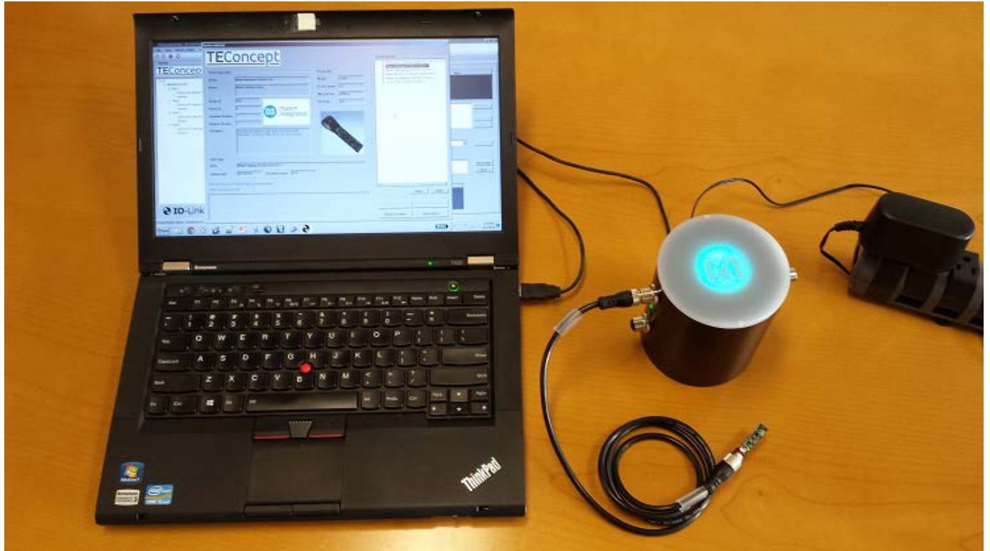
Figure 2. MAXREFDES79# system connected and running.
