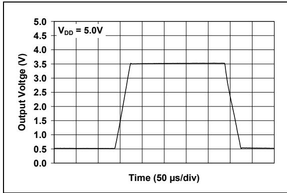
FIGURE 2-25: Large-signal, Non-inverting Pulse Response.
