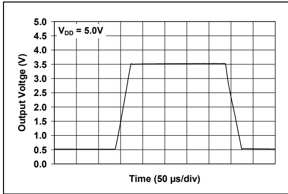
FIGURE 2-25: Large-signal, Non-inverting Pulse Response.
