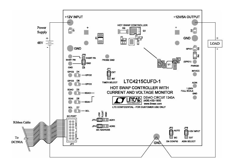
Figure 4. Proper Measurement Equipment Setup
