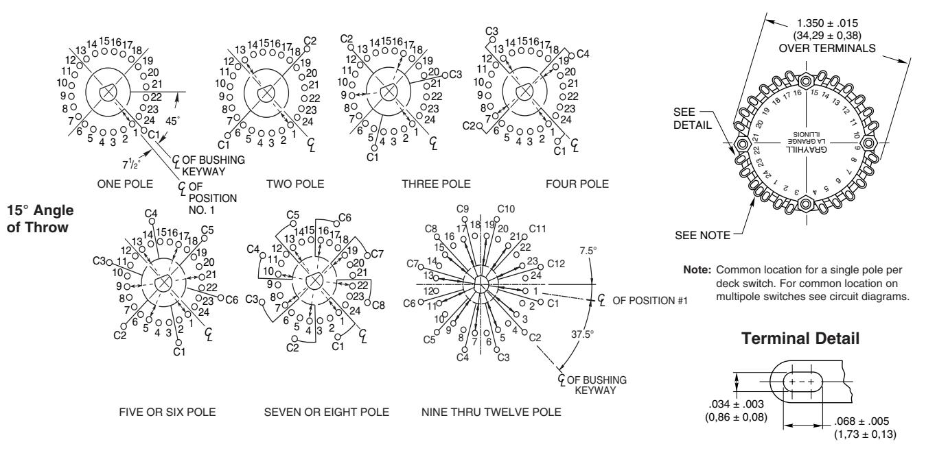
**CIRCUIT DIAGRAMS: Series 59****Switch is Viewed From Shaft End and Shown in Position No. 1**
