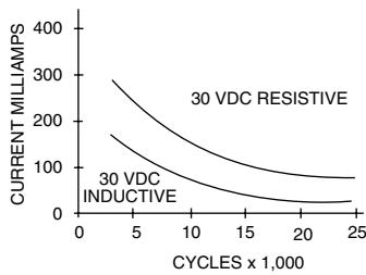
Curve data based on test data conducted at sea level, 25°C and relative humidity. Cycle equals 360° rotation and 360° return. Cycling rate is 10 cycles per minute. The curves shown are typical load life curves for a Series 53M, 57M and 59M Rotary Switch. They show the number of cycles of rotational life that can be expected for the voltages, currents and
