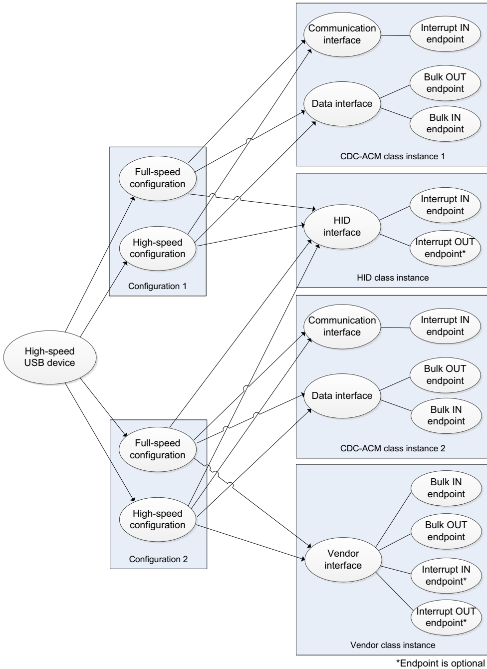
Figure 5-2 Complex Composite High-Speed USB Device Structure
