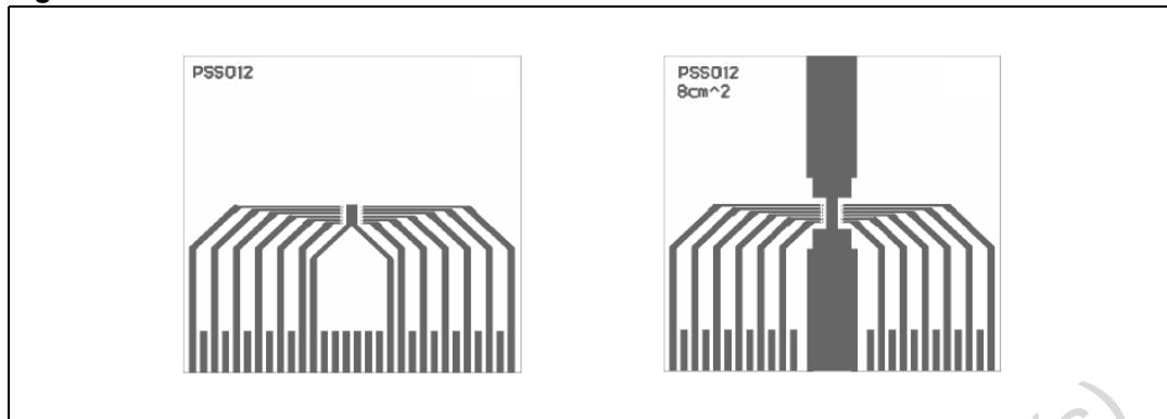
Note: Layout condition of  $R_{th}$  and  $Z_{th}$  measurements (PCB FR4 area = 78 mm x 78 mm, PCB thickness = 2 mm, Cu thickness=35  $\mu$ m, Copper areas: from minimum pad lay-out to 8  $cm^2$ ).
