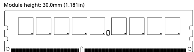
Figure 2: 240-Pin UDIMM (MO-269 R/C D1) PCBs 1483 & 1568
