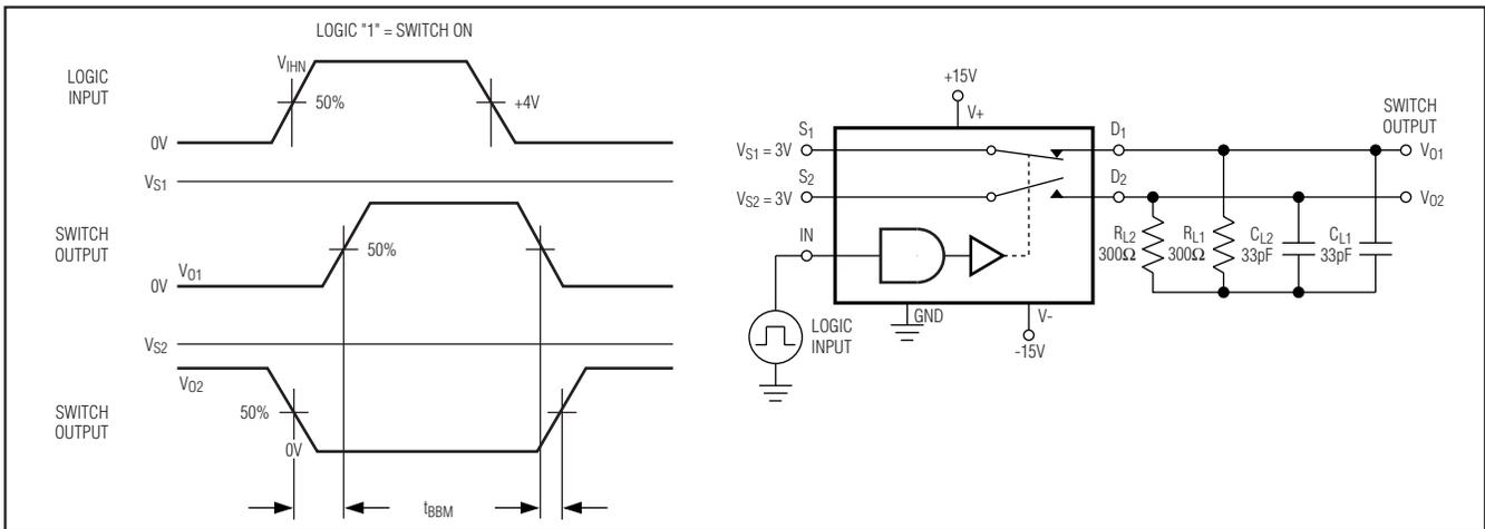
Figure 2. Break-Before-Make Time Test Circuit SPDT (DG301(A), DG303(A))
