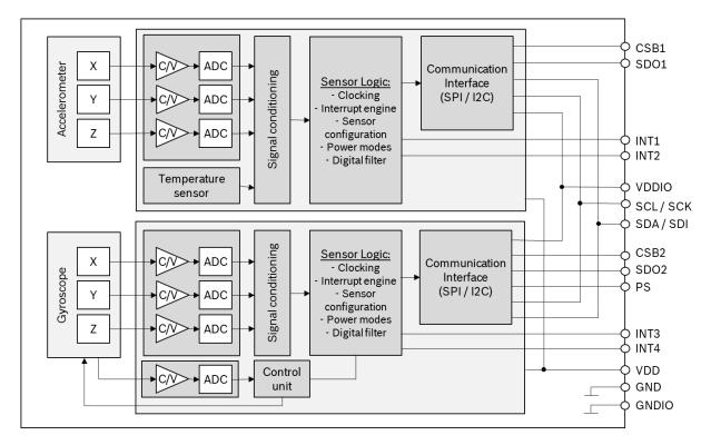
Figure 1: Block diagram of BMI085
