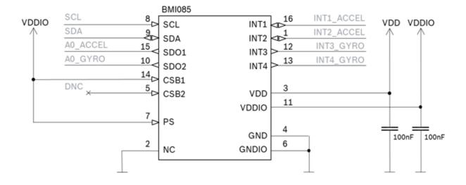
Figure 9: I<sup>2</sup>C connection
