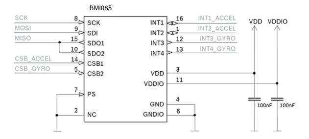
Figure 8: SPI connection
