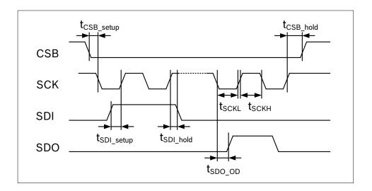
Figure 2: SPI timing diagram
