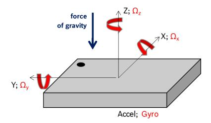
Figure 11: Orientation of sensing axis
