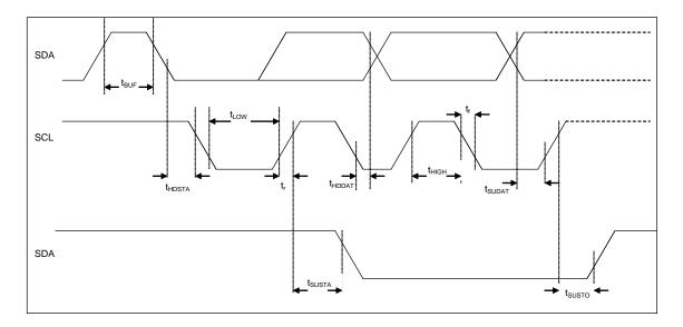
Figure 3: I<sup>2</sup>C timing diagram
