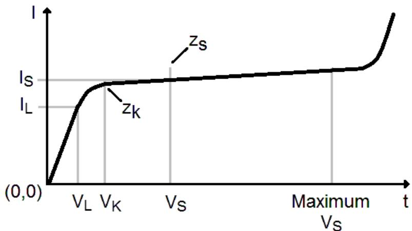
**FIGURE 1 – CURRENT-REGULATOR CHARACTERISTICS**
