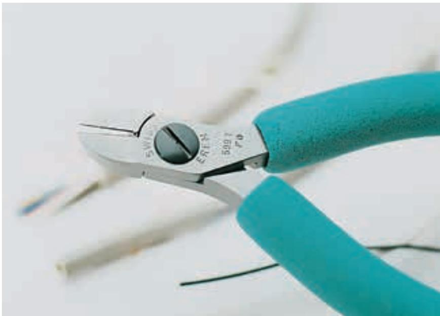
The 599TFO has wear resistant tungsten carbide cutting edges and all round capability. It is able to cut Vectran™ braided wires, fibre optics, Kevlar® and small stainless steel braids and wires.
