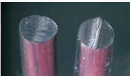
+ **Erem cut Super full flush: perfect flush cut** Standard cut „Super full flush“
