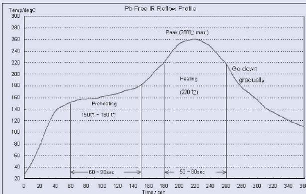
1. Preheating shall be fixed at 150~180°C for 60~90 seconds.
